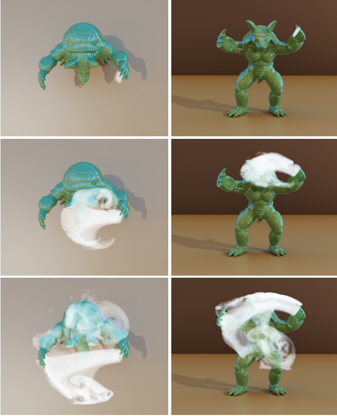
Fig. 10: Smoke flow through armadillo. We set a smoke source on Armadillo’s left hand, and with the wind speed, the smoke is drifting to its right hand. Smoke will pass through Armadillo’s head and ears along the way and generate vortices. This example also uses the spherical shell space as the simulation domain, and the geometry of the armadillo is superimposed on a base sphere as terrain.
