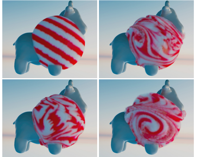
Fig. 12: A tiny cow geometry is imported as terrain. The cloud around the cow is initialized by a divergence-free velocity, due to our geometric-aware 3D solver, the cloud could flow around the tiny cow and climb along the surface.
